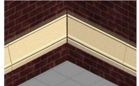
A mitered corner is another option of connecting your parts together.
