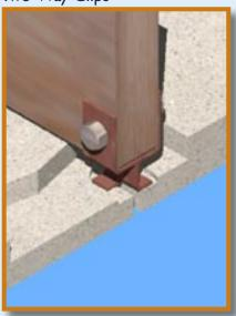
Two-Way Clips require inset grooves to protect the stone from cracking.
