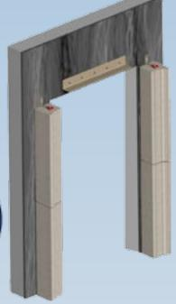
Place the straight leg sections into position. Make sure it is Level. Mark and drill the holes for the steel setting pin. Utilize spacers to achieve the correct mortar joint spacing.
