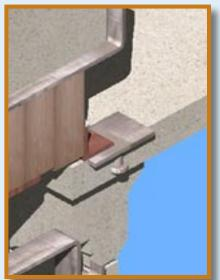
Embedded weld plate inserts support the stone structure.
