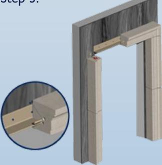
The horizontal pieces of the surround can be held in place with steel lintels and tapcon screws. Wire and pin are used to keep the stone from tipping. Drill a pin hole to secure the facing stone of the horizontal section.
