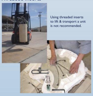
Threaded inserts can be added in the manufacturing process to attach the stone to other structures.
