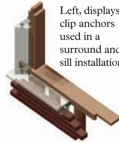
Left, displays clip anchors used in a surround and sill installation.
