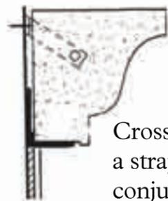
Cross section shows a strap anchor in conjunction with a steel lintel.
