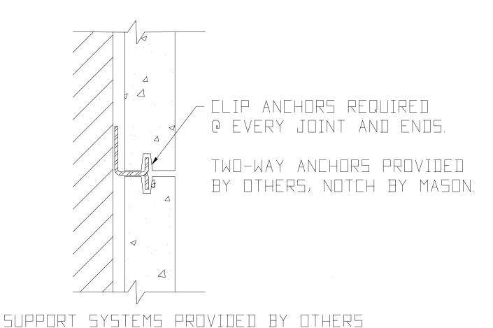
ATTACHMENT OF STACKED PANELS TO SURFAL WITH 2-WAY STRAP
