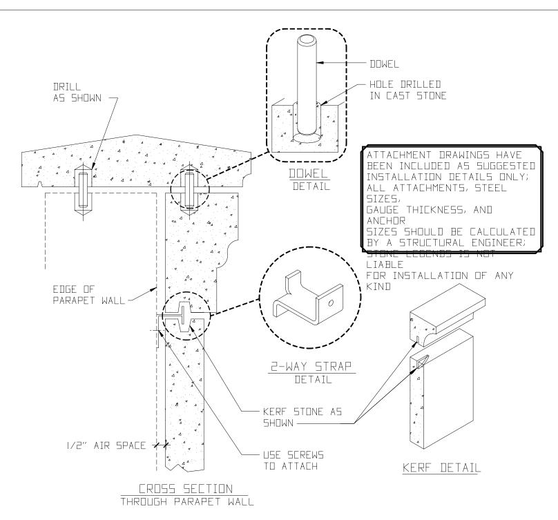
ATTACHMENT OF PARAPET CAP TO ENTABLATURE & PANEL
