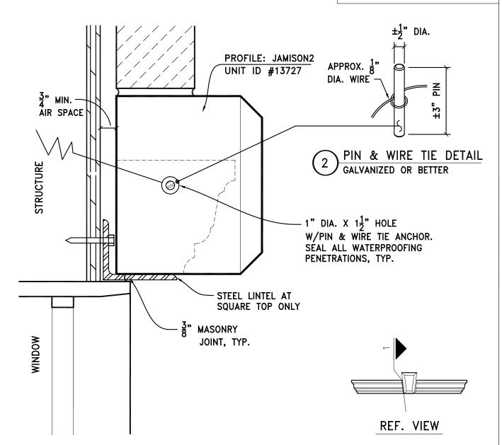
CAST STONE LINTEL ATTACHMENT AT MASONRY VENEER WITH PIN & WIRE TIE ANCHOR
