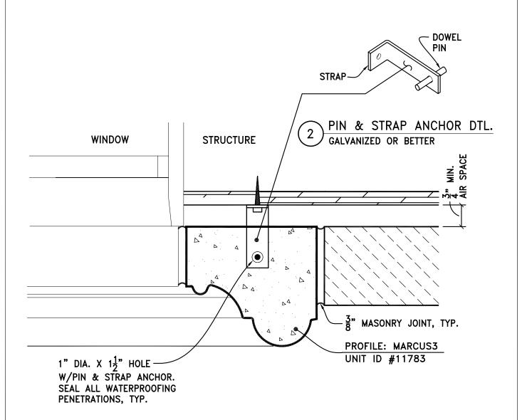
CAST STONE JAMB ATTACHMENT AT MASONRY VENEER WITH PIN & STRAP ANCHOR
