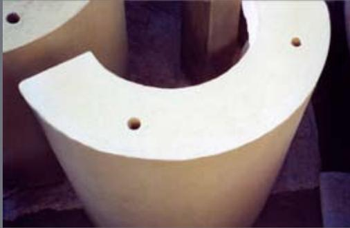
Column sections are aligned with pre-cast holes and pins.
